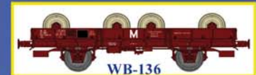
PLAT OCEM 29 Ep.IV, Porte Essieux OCEM 29 flatcar Era IV - Axles-transport - Rollbearing wheelboxes
