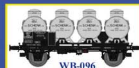
Porte-Container Ep.III, 4 x Citernes rondes "SCHENK" Flat Car, Spoked wheels, era III - 4 round tanks "SCHENK"
