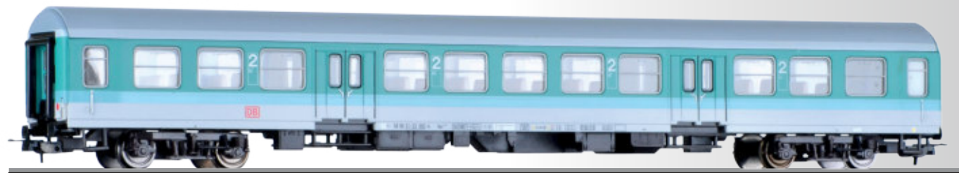
Reisezugwagen 2. Klasse By 407, Bauart Halberstadt, der DB AG 2nd class passenger coach By 407, type Halberstadt, of the DB AG
