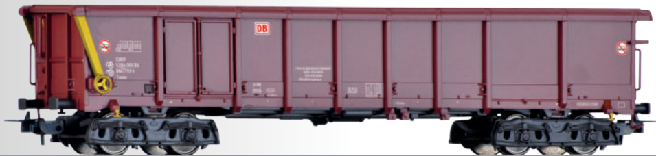
Rolldachwagen Taems der DB AG Sliding roof car Taems of the DB AG
