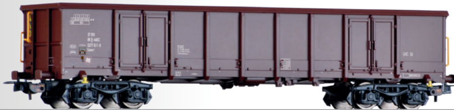
Offener Güterwagen Eanos der AAE Cargo Open car Eanos of the AAE Cargo
